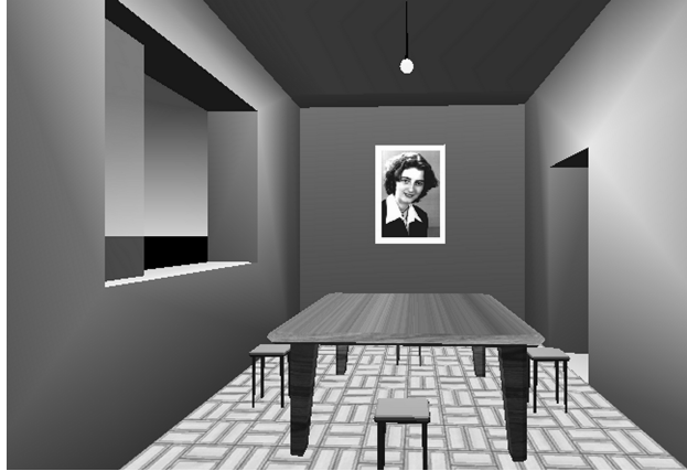
Figure 7 Perspective view of a CAD of a room, rendered with shading, textures, and transparency.
